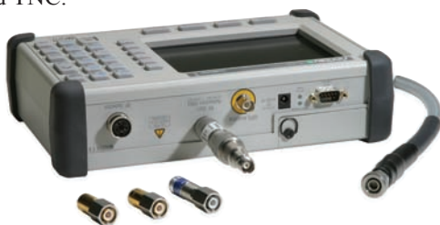
Adapt to a variety of coaxial connectors.
